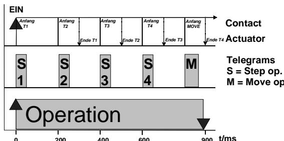
If the button is held after all step commands have been sent a continuous command (move) is sent to the bus in accordance with the set time (factor x base) that controls the actuators into the continuous mode.
