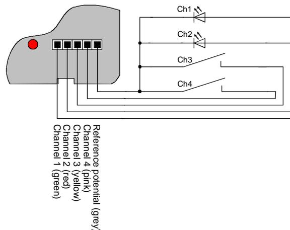
Example of universal interface used with 2 inputs and 2 outputs
