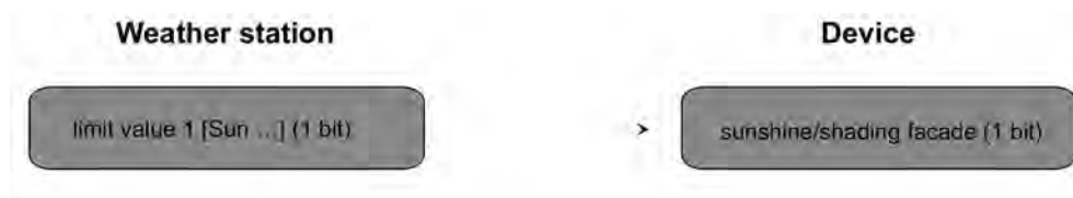
picture 25: Programming of the communication objects for application example I.
