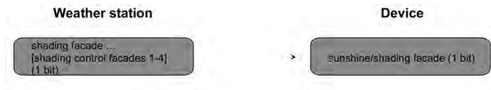
picture 26: Programming of the communication objects for application example II.
