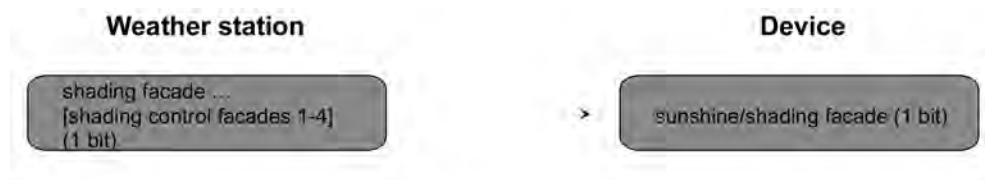
Figure 26: Programming of the communication objects for application example II.
