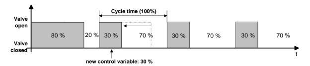
Before receipt of the new manipulated variable (30 %) the old setpoint (80 %) was active. The new manipulated variable is received during the opening phase of the valve. At this point in time the actuator recognises that it is still possible to cut short the opening phase so that it corresponds to the new manipulated variable (30 %). The cycle time is unchanged by this procedure.
