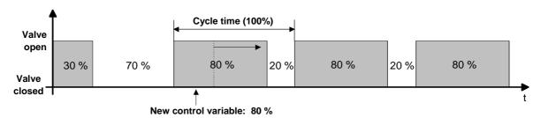
Before receipt of the new manipulated variable (80 %) the old setpoint (30 %) was active. The new manipulated variable is received during the opening phase of the valve. At this point in time the actuator recognises that it is still possible to extend the opening phase so that it corresponds to the new manipulated variable (80 %). The cycle time is unchanged by this procedure.
