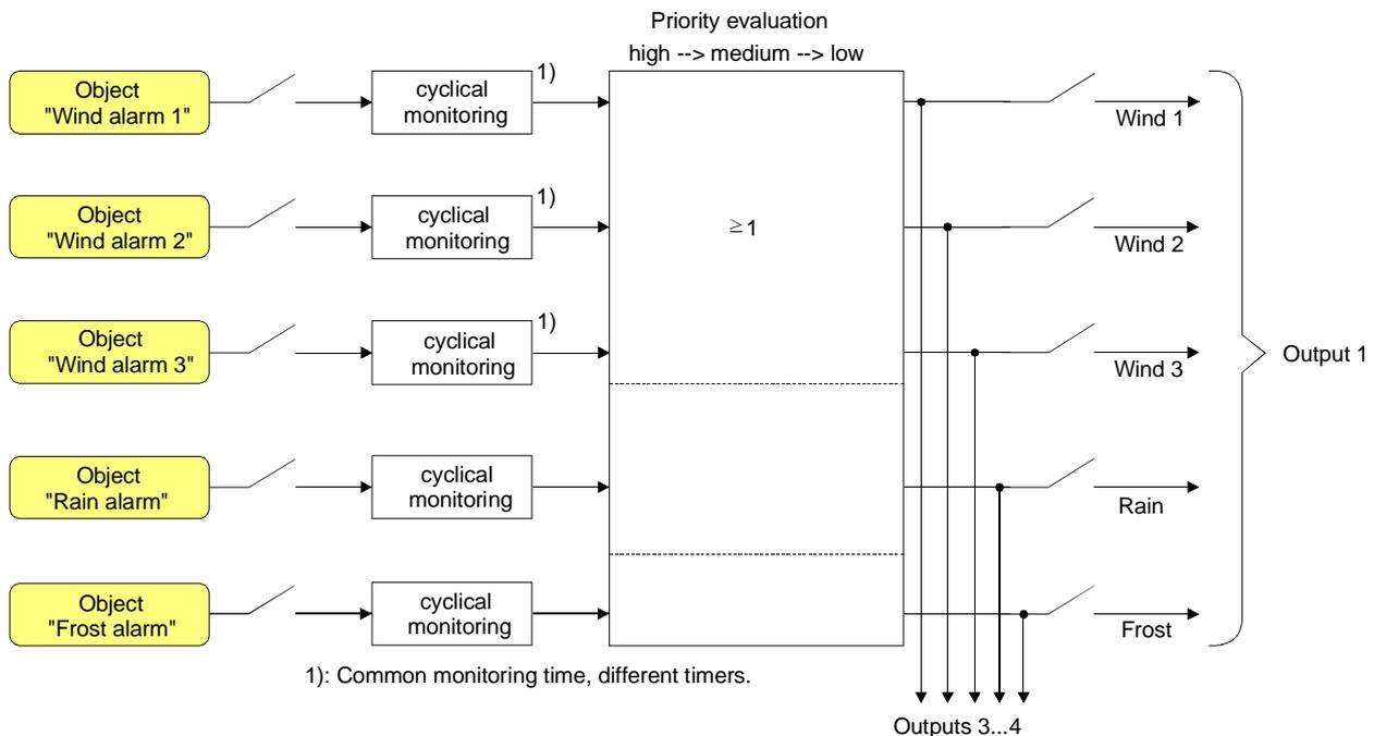
Fig. 8: Function diagram of the safety function
