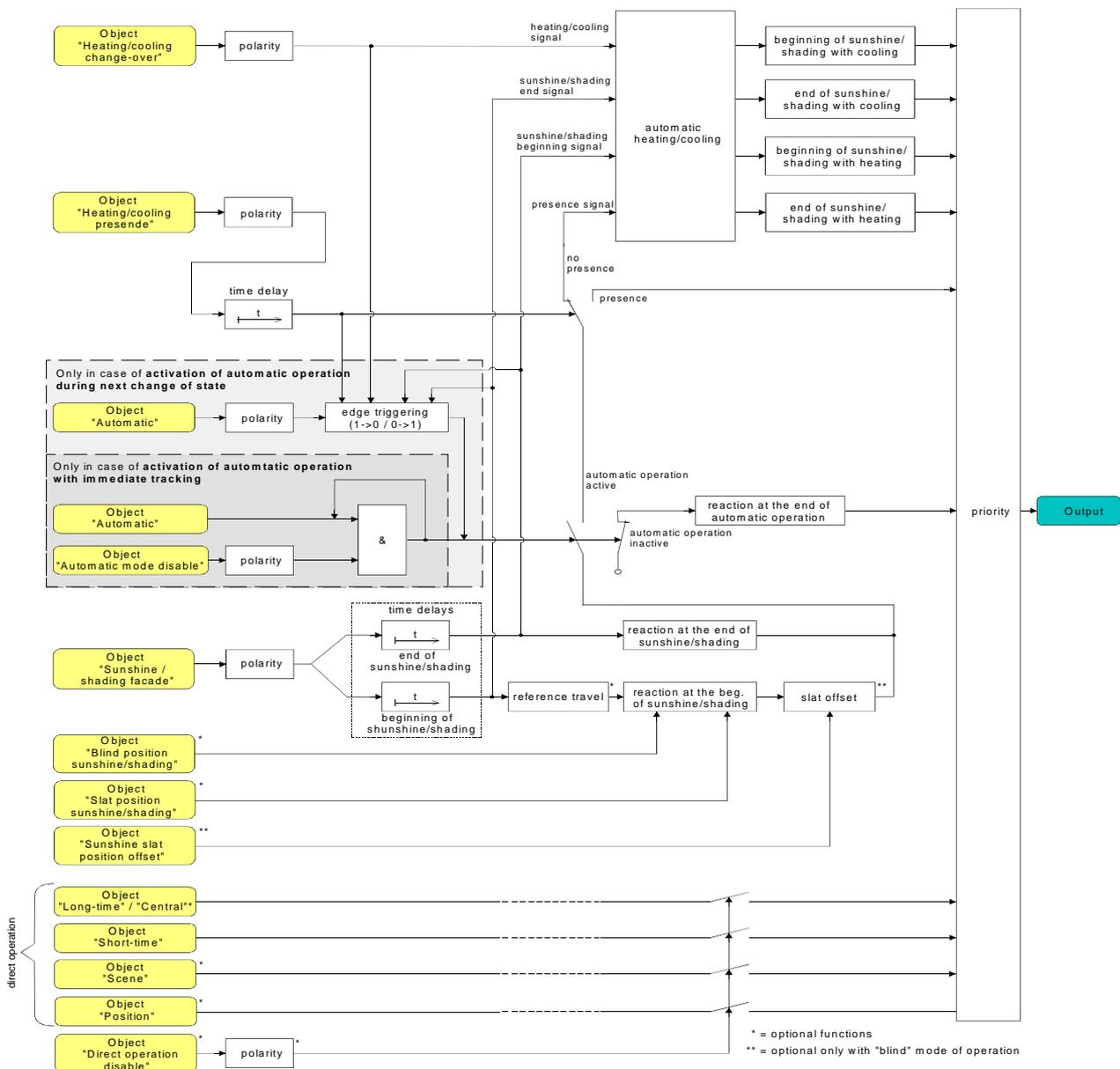
Fig. 29: Schematic diagram of automatic heating/cooling
