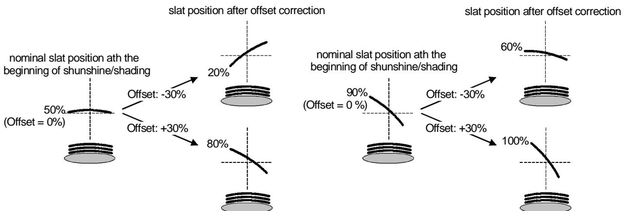
Fig. 22: Functional principle of slat offset
