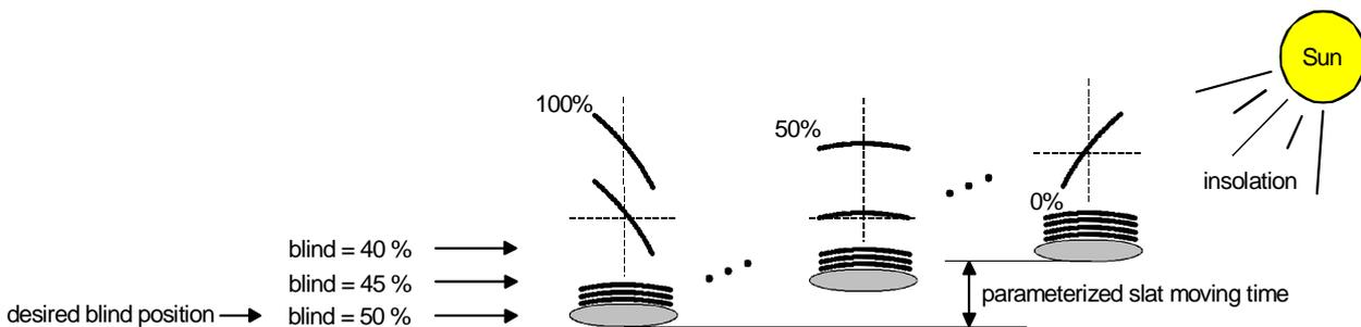
Fig. 13: Example of slat positioning affecting the position of the blind (typical of slat type 1; analogous reaction for type 2)
