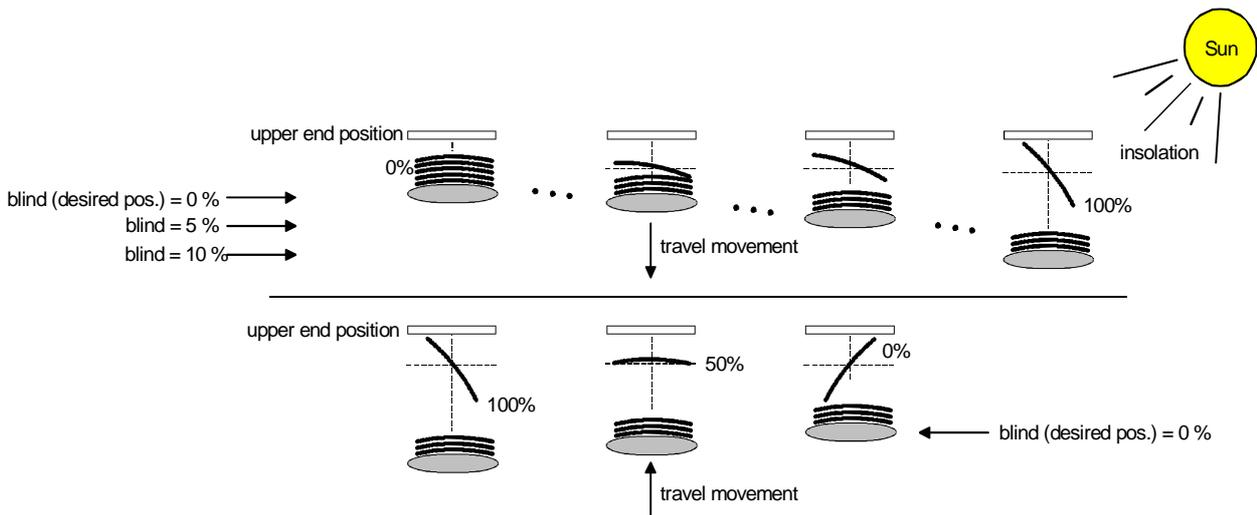
Fig. 14: Example of slat positioning with the blind in upper end position (typical of slat type 1)
