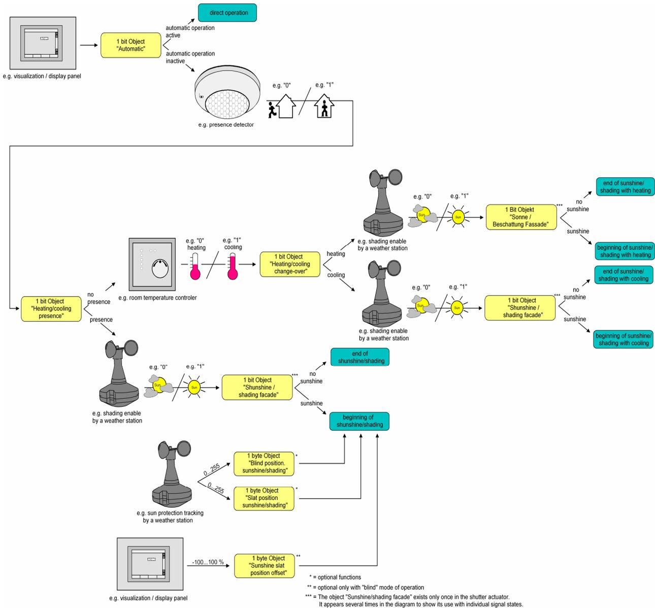
**Fig. 28: Schematic diagram of the automatic heating/cooling system**
