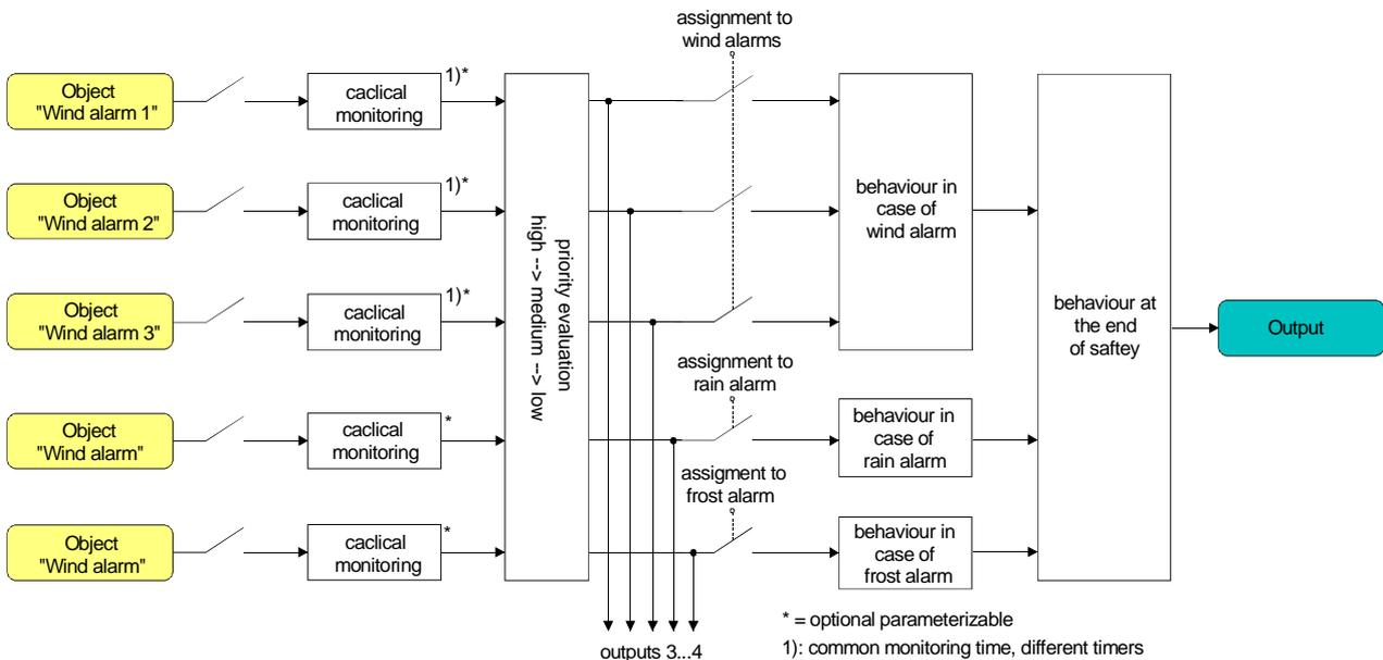
Fig. 16: Function diagram of channel-oriented safety functions
