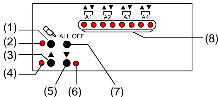
Fig. 6: Controls and indicators for manual control
