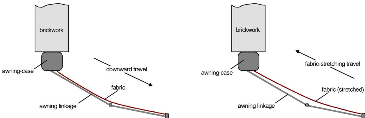
Fig. 30: Fabric-stretching in an awning
