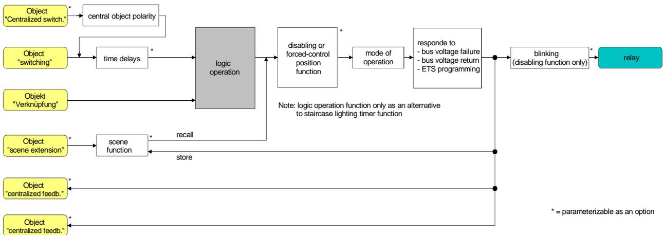
Fig. 19: Functional diagram of the logic function
