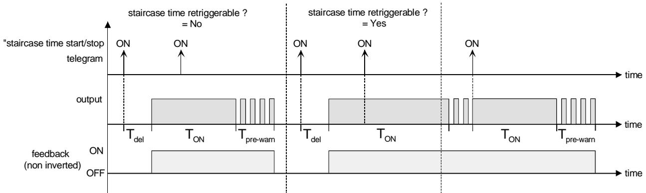
Fig. 11: Switch-on behaviour of the staircase function
