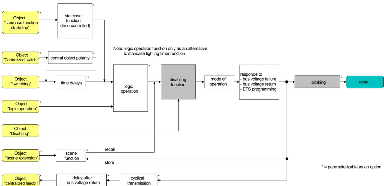
Fig. 17: Functional diagram of the disabling function
