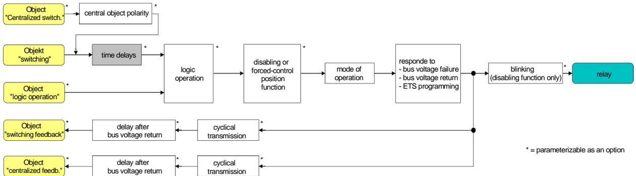
Fig. 9: Functional diagram of the time delays
