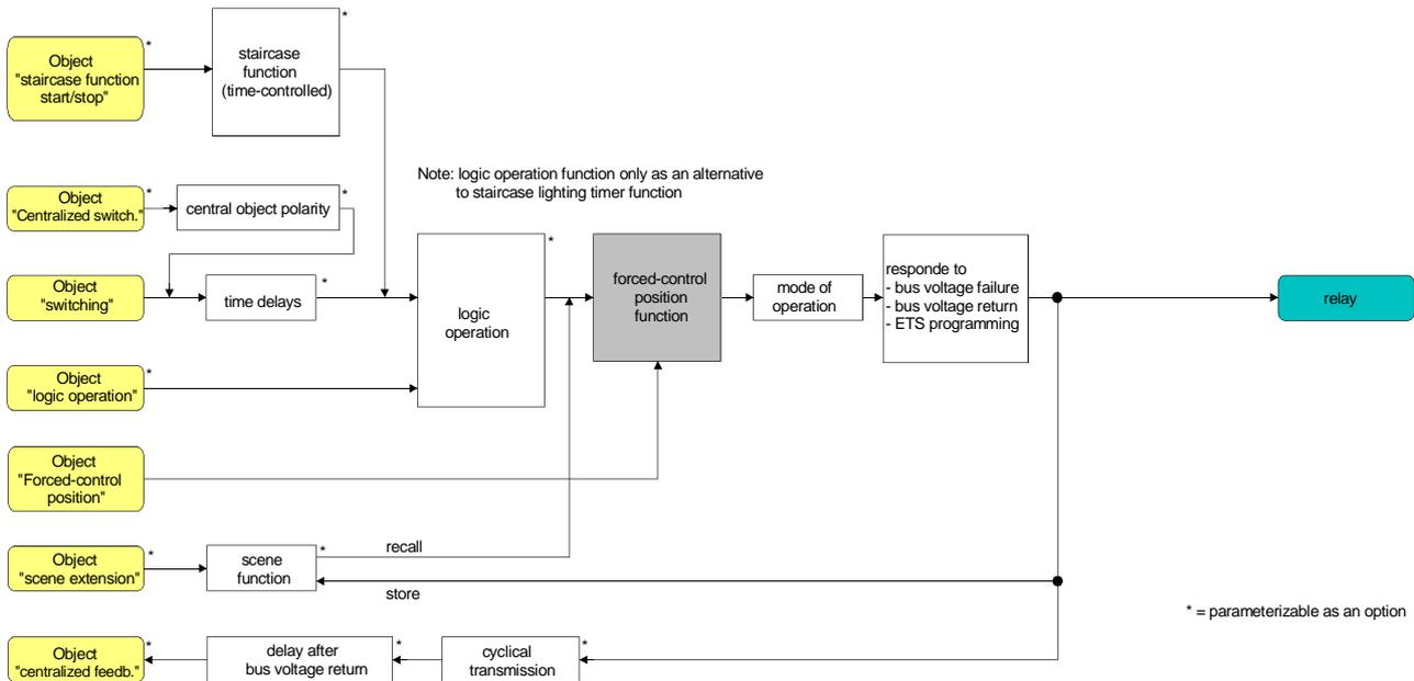
Fig. 18: Functional diagram of the forced-control position function
