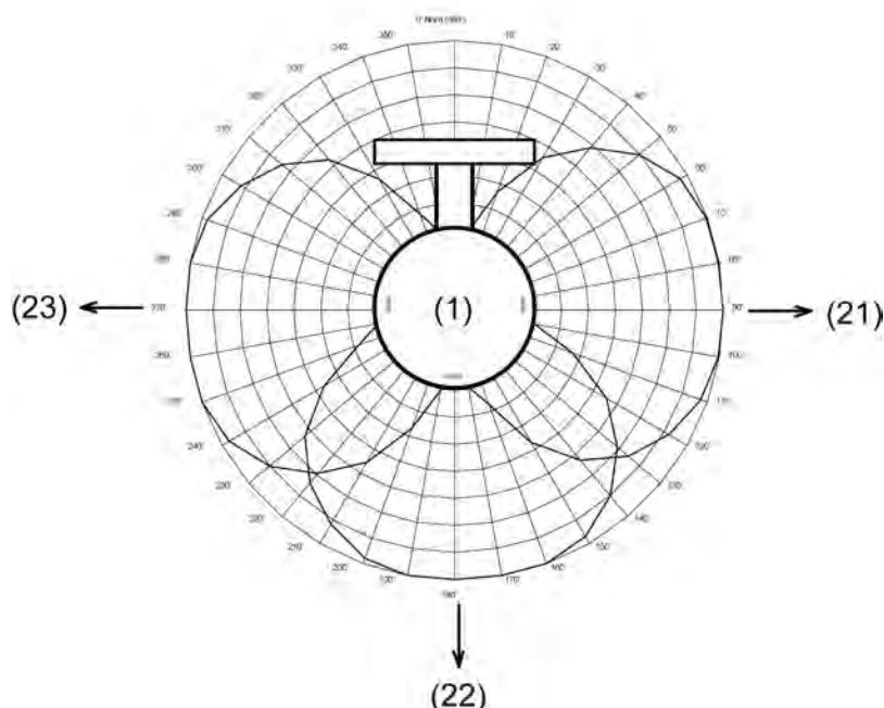
picture 4: Orientation of the weather station
