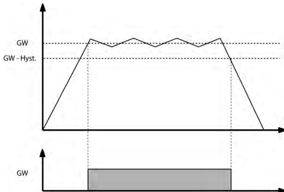
picture 13: Frequency of switching with hysteresis parameterised.
