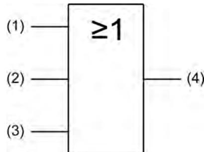
picture 10: Logic for controlling the wind alarm
