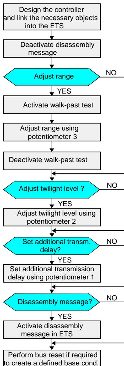
Once all devices (for instance masters and slaves in a project) have been configured and individually commissioned, it is recommended that a bus reset is performed, to create a defined base condition.
