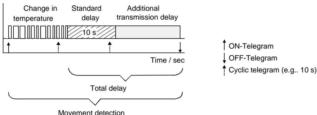
Messages can be sent for the start and the end of a movement detection. During a movement detection the controller is always in brightness-independent mode, i.e. it will trigger the start of the total delay count-down at each new movement detection, irrespective of the ambient brightness.
