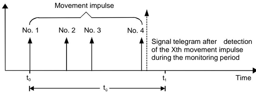
⇒ After detecting the 4th movement impulse ( $x = X$ ) within the monitoring period  $t_{\bar{u}}$ , a “report message after detecting the Xth movement impulse” is sent in accordance with the parameterisation.
