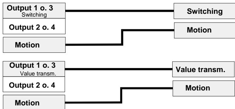
Switching the twilight level of the slaves on and off, where not parameterised to brightness-independent, is done by linking the output objects. An object value > 0 at the start of the detection causes the twilight level (brightness-independent) to be deactivated, and an object value = 0 after the additional transmission delay has elapsed causes the twilight level (brightness-dependent) to be activated.
