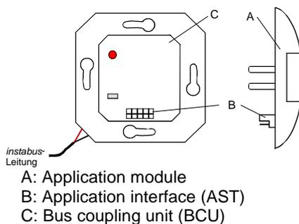
The application interface (B) of the application module must be underneath, otherwise the appliance will not function correctly.
