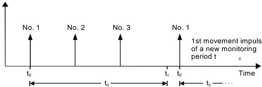
⇒ In the first monitoring period only 3 movement impulses ( $x < X$ ) were detected. It follows that no report message is triggered. After  $t_{\bar{u}}$  has elapsed the next movement impulse will be the first of a new monitoring period  $t_{\bar{u}}$ .
