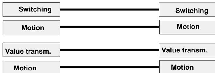
Switching the twilight level of the slaves on and off, where not parameterised to brightness-independent, is done by linking the output objects (object 0 or 1). An object value > 0 at the start of the detection causes the twilight level (brightness-independent) to be deactivated, and an object value = 0 after the additional transmission delay has elapsed causes the twilight level (brightness-dependent) to be activated.
