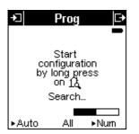
The Prog screen allows starting the learning phase of the products of the installation.
