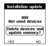
This function allows erasing from the project file the products which were detected, but not linked.
