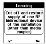
The RF section of an installation is identified with one single RF product. Switch a bidirectional RF product off and on again.
