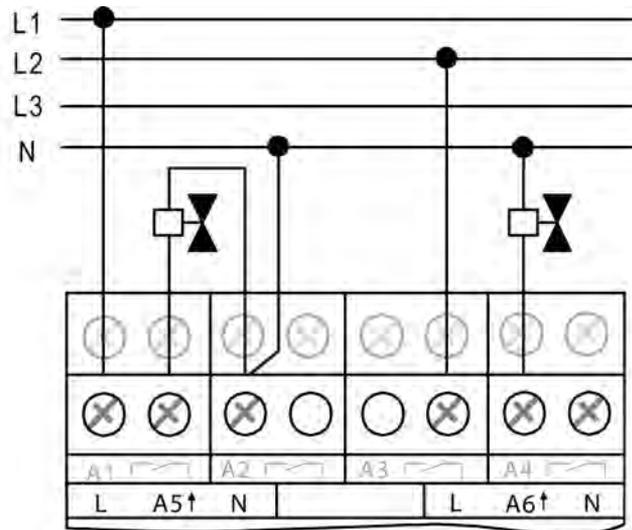
picture 5: Electrical connection for electrothermal valve drives
