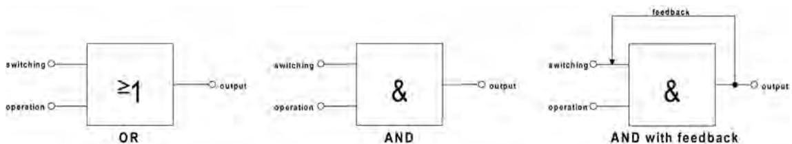
picture 27: Gating operations of the logic function
