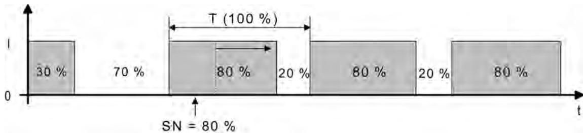
picture 62: Command value change e.g. from 30 % to 80 % during the opening phase of the valve
