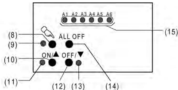
picture 7: Controls and indicators for manual control on the front panel of the device.
