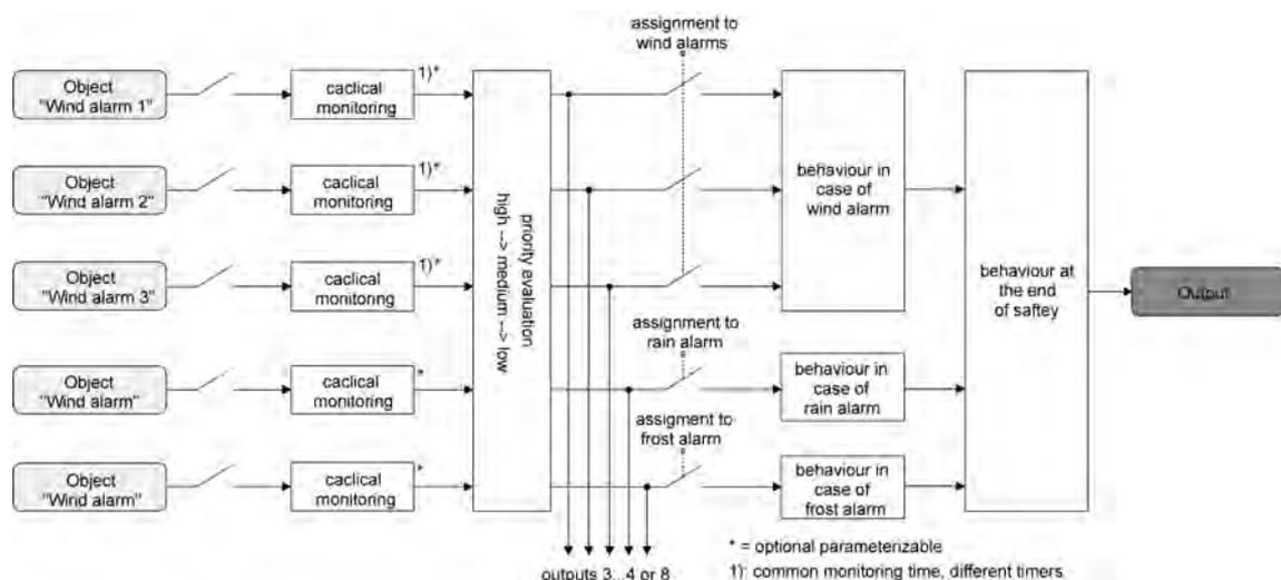
picture 36: Function diagram of channel-oriented safety functions
