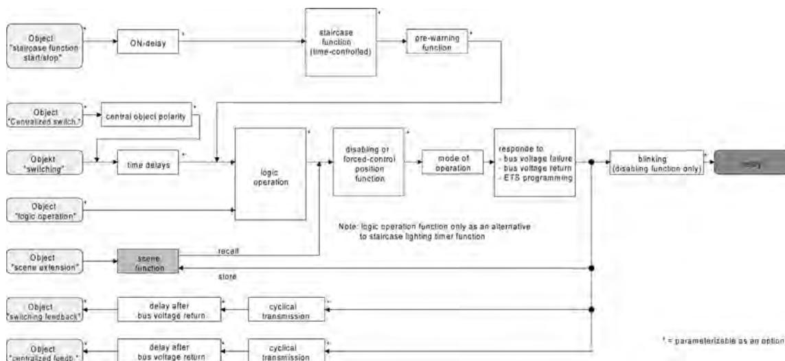
picture 22: Functional diagram of the scene function
