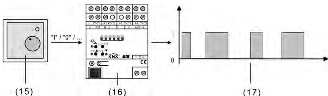
picture 56: Command value principle with switching command value
