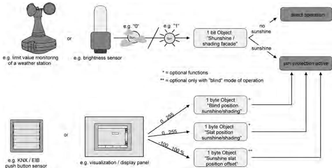
picture 38: Schematic diagram illustrating the simple sun protection configuration
