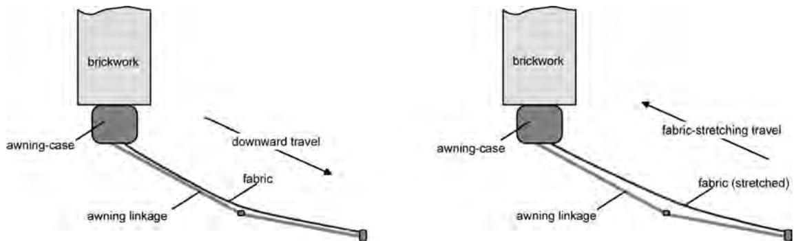
picture 50: Fabric-stretching in an awning
