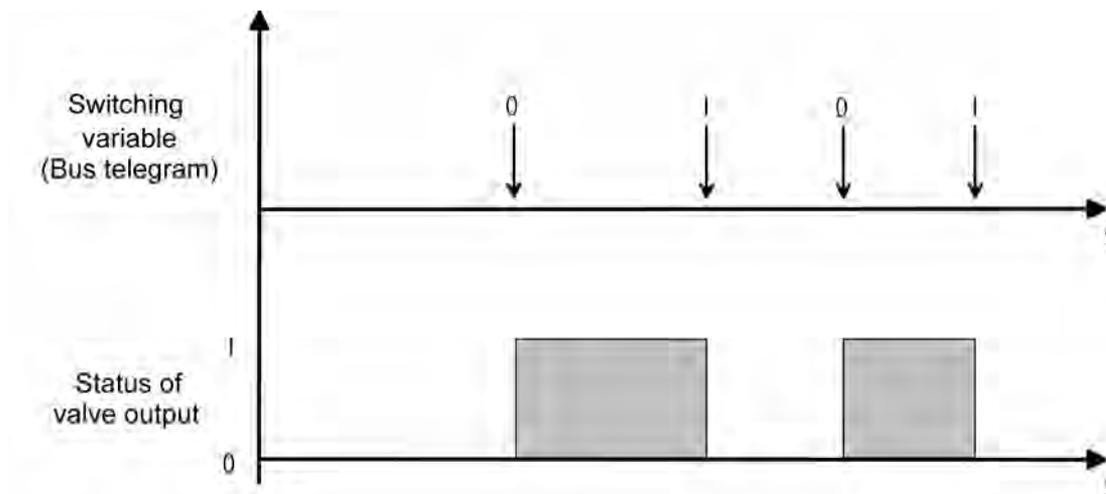
picture 53: Conversion of a switching command value into an output signal with valve drives that are open when deenergized (example)
