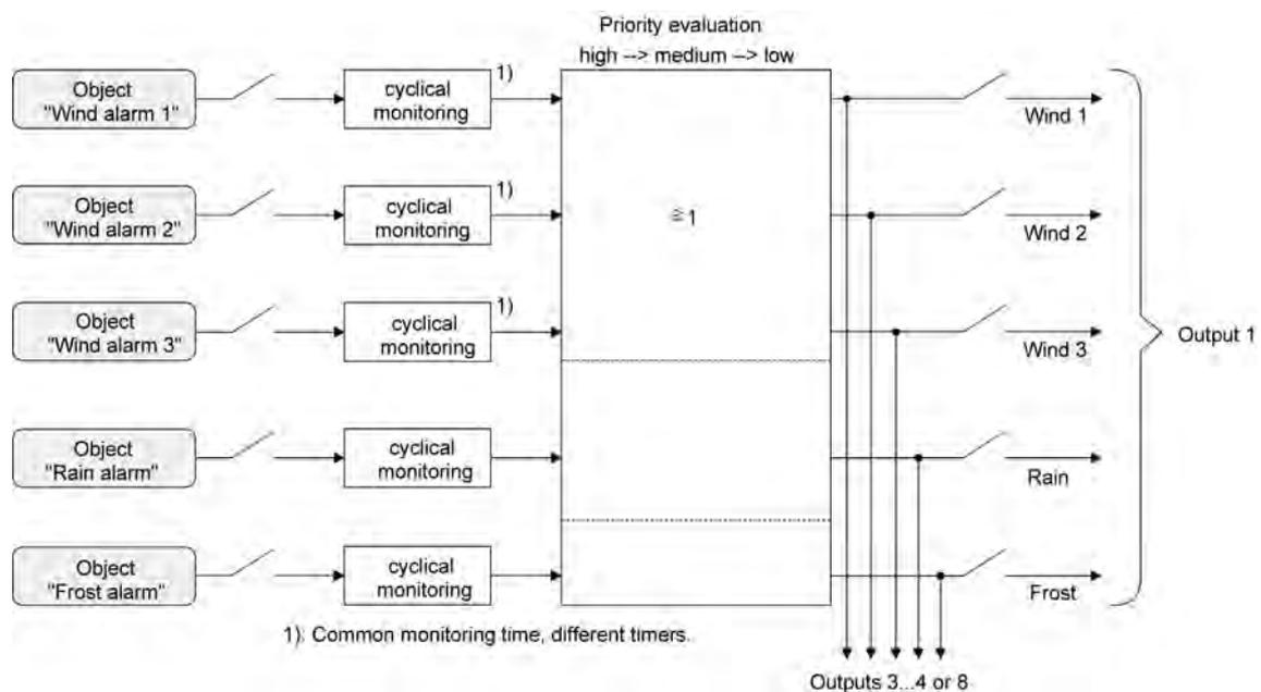
picture 13: Function diagram of the safety function
