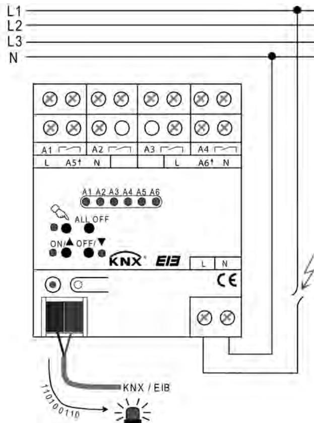
picture 8: Monitoring of the mains voltage
