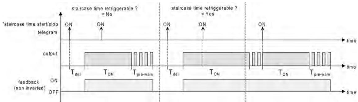
picture 18: Switch-on behaviour of the staircase function
