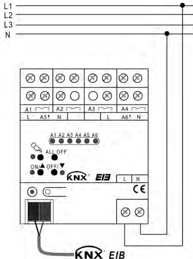
picture 2: Electrical connection of mains voltage
