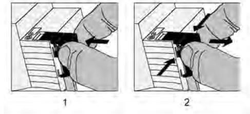
picture 6: Installing / removing the protective cap for the bus connection
