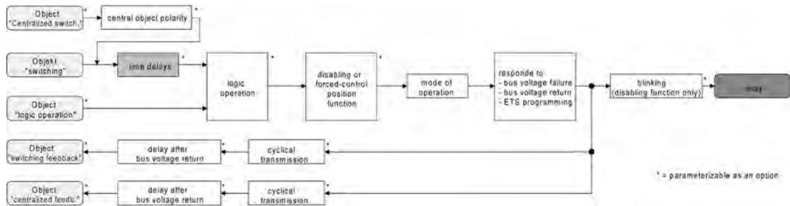
picture 16: Functional diagram of the time delays
