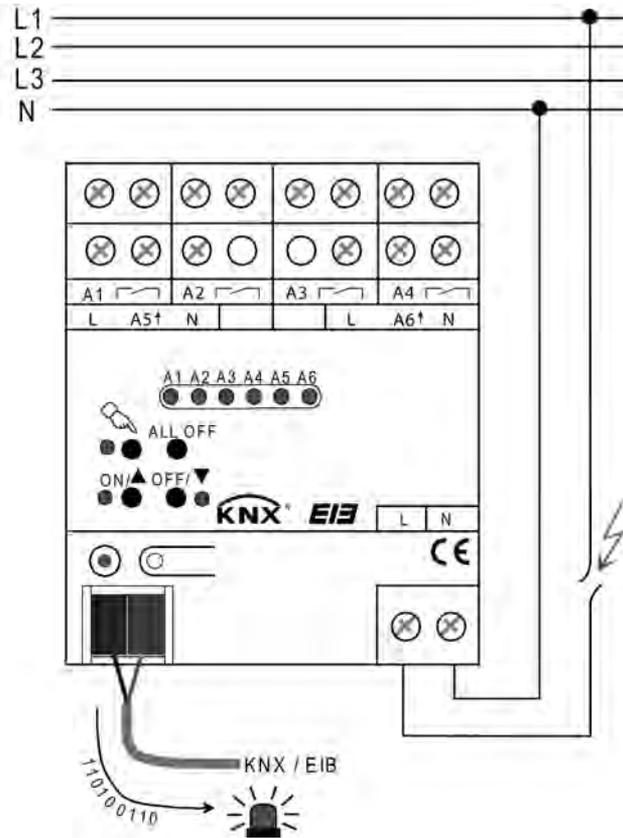
picture 8: Monitoring of the mains voltage
