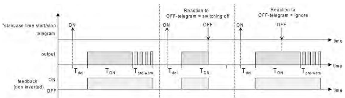
picture 19: Switch-off behaviour of the staircase function
