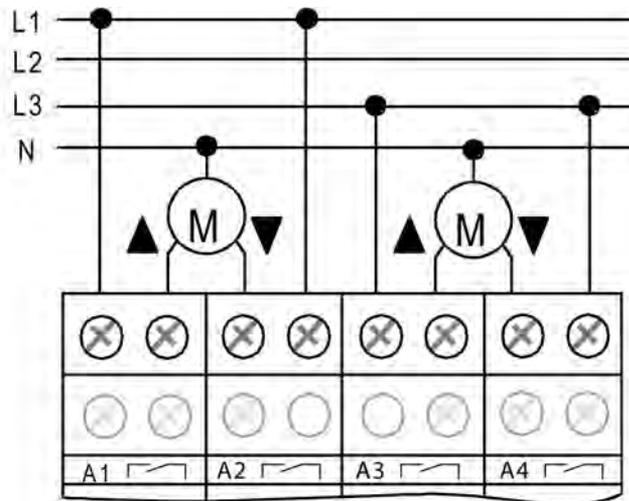
picture 3: Electrical connection for 230 V drives in blinds operation
