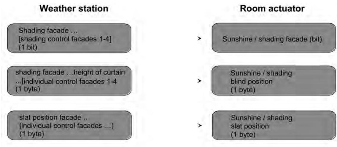
picture 46: Programming of the communication objects for application example IV
