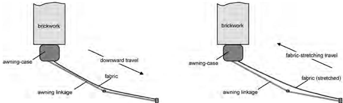
picture 50: Fabric-stretching in an awning
