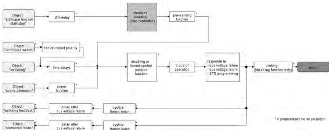
picture 17: Functional diagram of the staircase function
