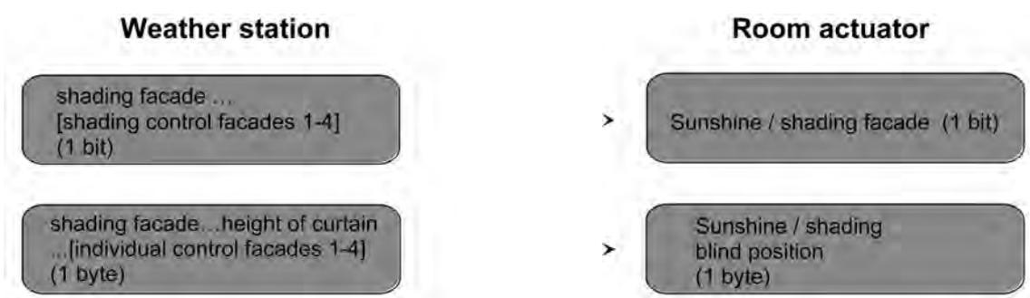
picture 47: Programming of the communication objects for application example V
