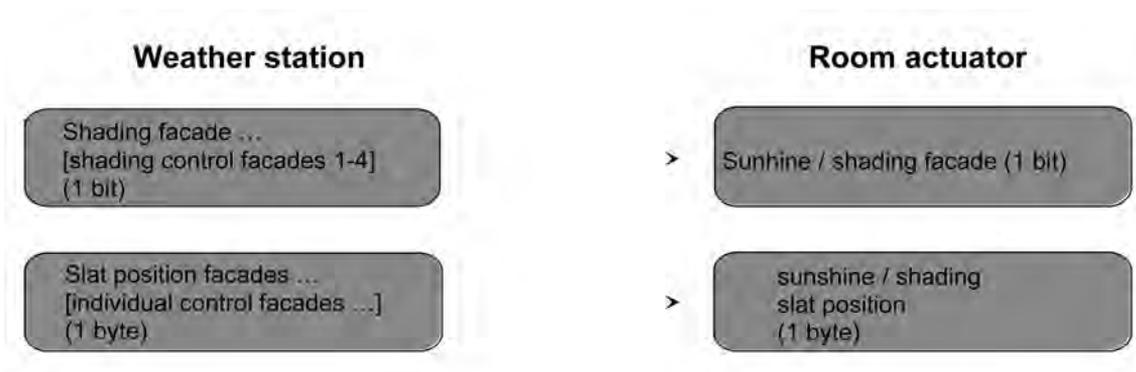
picture 45: Programming of the communication objects for application example III
