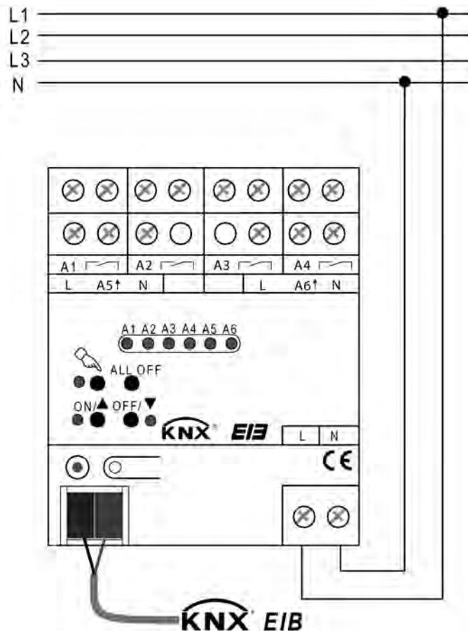
picture 2: Electrical connection of mains voltage
