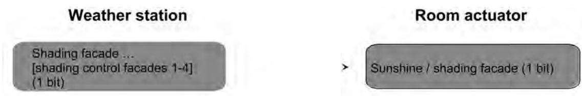
picture 44: Programming of the communication objects for application example II
