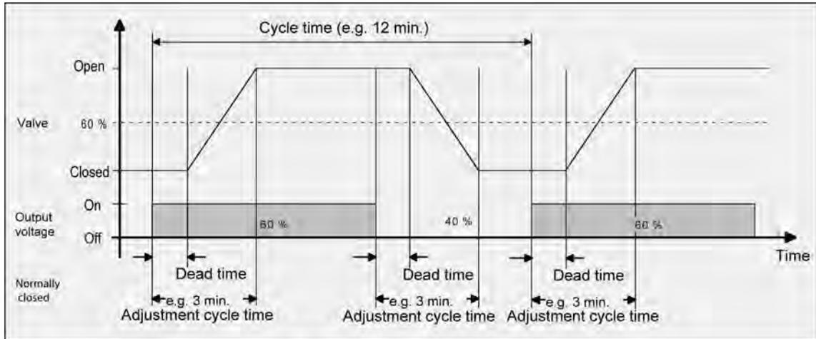
picture 65: Idealised curve of the valve stroke: example for a command value of approx. 60 % for a valve closed when deenergized
